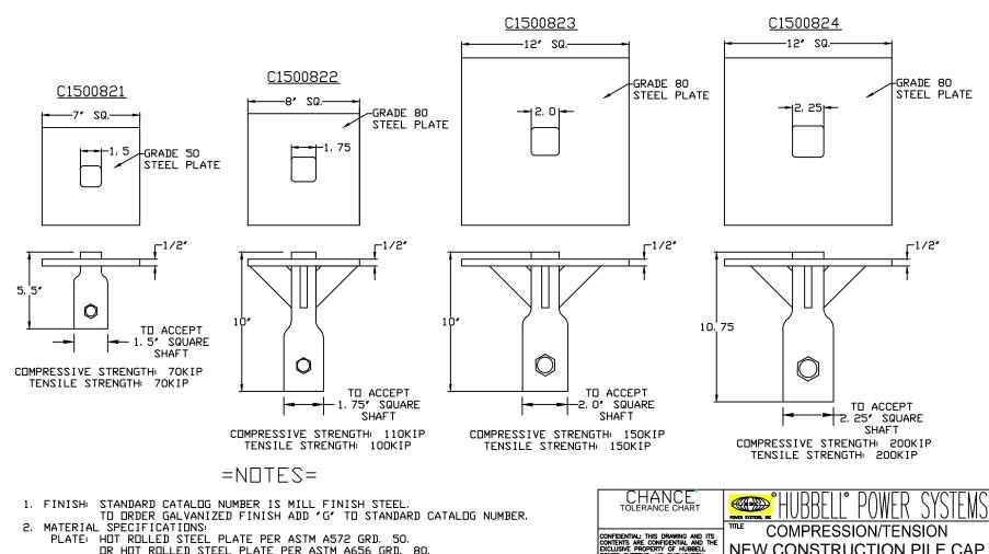
OR HOT ROLLED STEEL PLATE PER ASTM A656 GRD. 80. SUCKET: ROUND CORNER SQUARE STEEL BAR PER TT-76 BOLT: 3/4" HEX HEAD BOLTS PER ASTM A325 TYPE 1. 7/8", 1-1/8", AND 1-1/4" HEX HEAD BOLTS PER ASTM A193.
